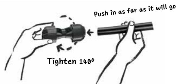
**C** Now connect the elements. Push the pipes approx. 6 cm into the connecting part over the O-ring, creating a water-tight connection. Caution: a sealing ring is positioned after approx. 4 cm. At this point, push the pipe further into the hole.
