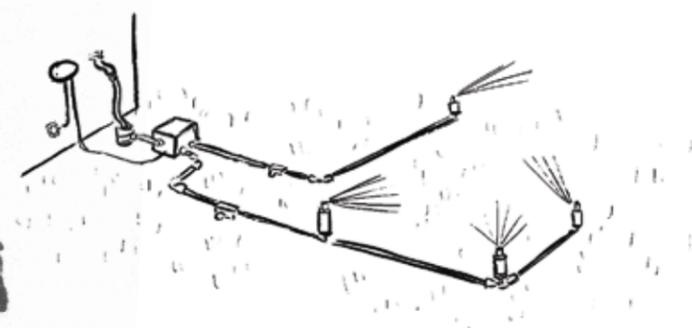
**E Important! Now check that your sprinkler system is watertight.** To check this, carry out a test run before you lay the system underground. If the sprinkler system is watertight, continue to Step F. If it is not watertight, check to see if the pipes are actually placed as far as they will go into the coupler.
