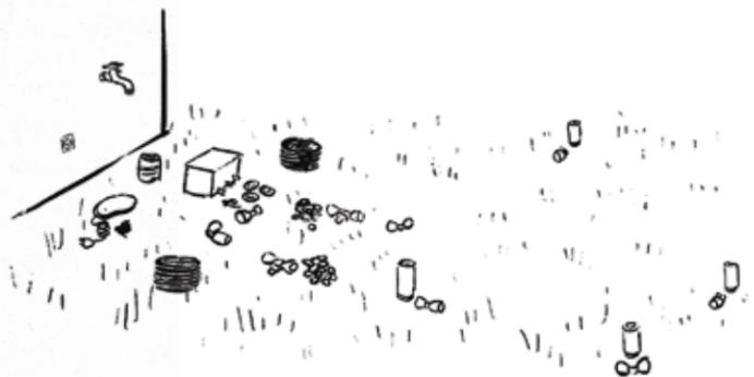
**A** Lay out all the parts in your garden in accordance with the plan. When doing so, start at the beginning of your watering system.
