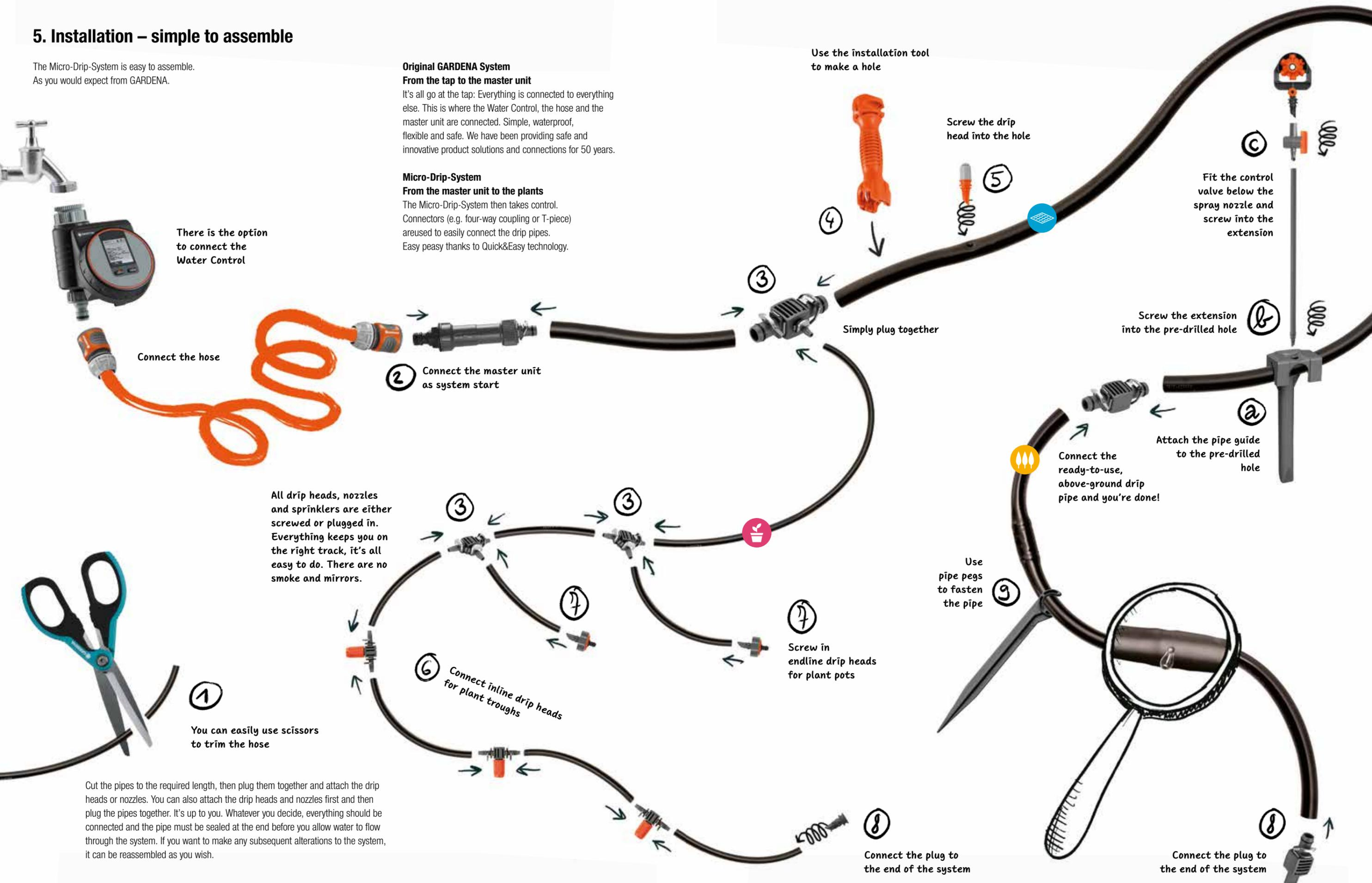
Cut the pipes to the required length, then plug them together and attach the drip heads or nozzles. You can also attach the drip heads and nozzles first and then plug the pipes together. It's up to you. Whatever you decide, everything should be connected and the pipe must be sealed at the end before you allow water to flow through the system. If you want to make any subsequent alterations to the system, it can be reassembled as you wish.
