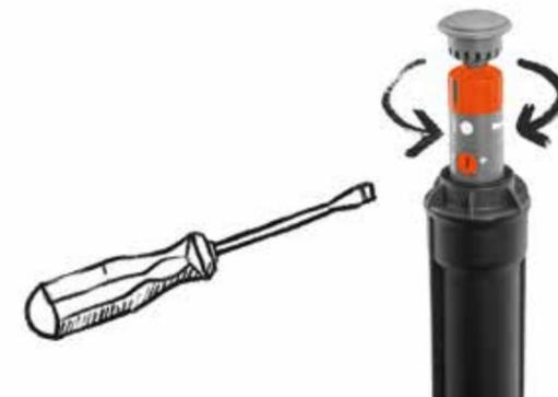
**D** Now adjust the spray direction, the sectors and the reach on the sprinkler. Simply use a screwdriver to turn the upper screw. This will allow you to regulate the range.
