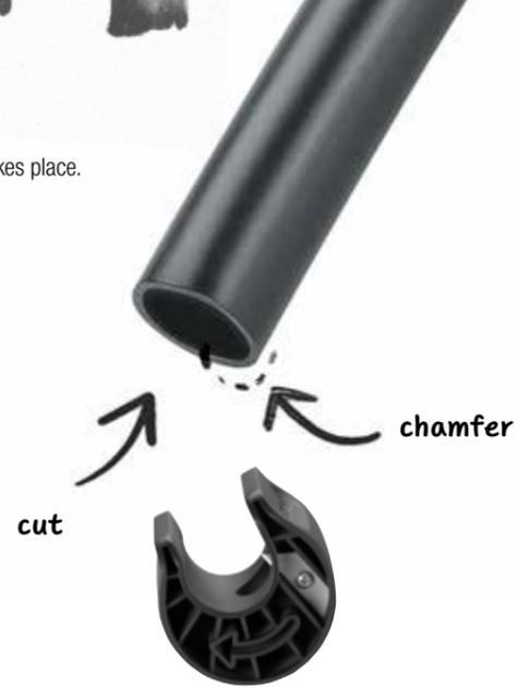
**B** Cut the pipes to the correct length in accordance with the plan. Make sure that no soil enters the pipeline. If necessary, chamfer the pipe, i.e. remove any dirty cut edges. For straight pipe cuts in just one turn, use the GARDENA Pipe Cutter.
